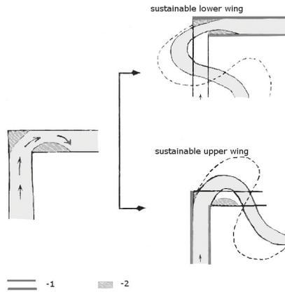
Figure 3. The formation and development of a new skewed meander at the site of a steep bend of the river with a stable lower and upper wings: 1-a relatively stable straight-line insertion; 2- an eddy zone
