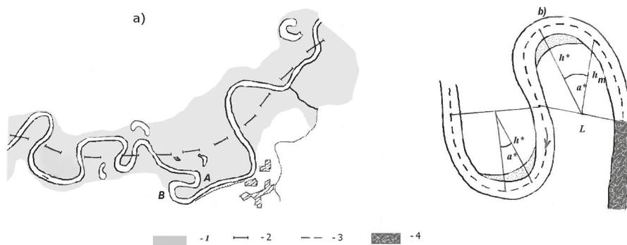
Figure 1. Example of the location of skewed meanders (A, B) on river Psel (a); morphological parameters of bed with skewed meanders (b): 1- floodplain; 2-axis valley; 3-bed center line; 4 straight insert
