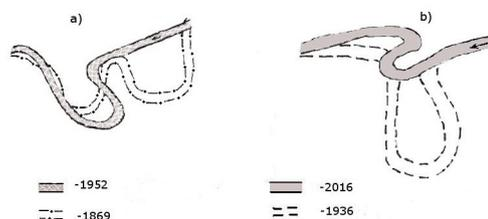
Figure 2. Formation of  $\gamma$ -shaped (a), and  $\Gamma$ -shaped (b) bend of the river, and the lowering of the adjacent bend after channel cut-off on the river Vorskla
