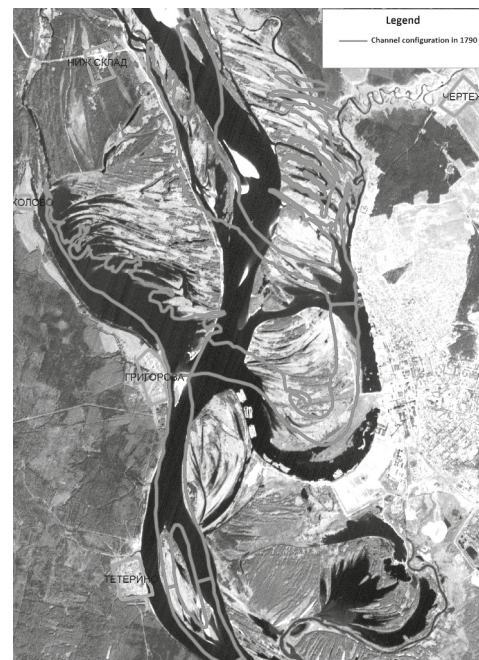
Figure 2. Change of a meandering channel to a relatively straight one at Solikamsk
