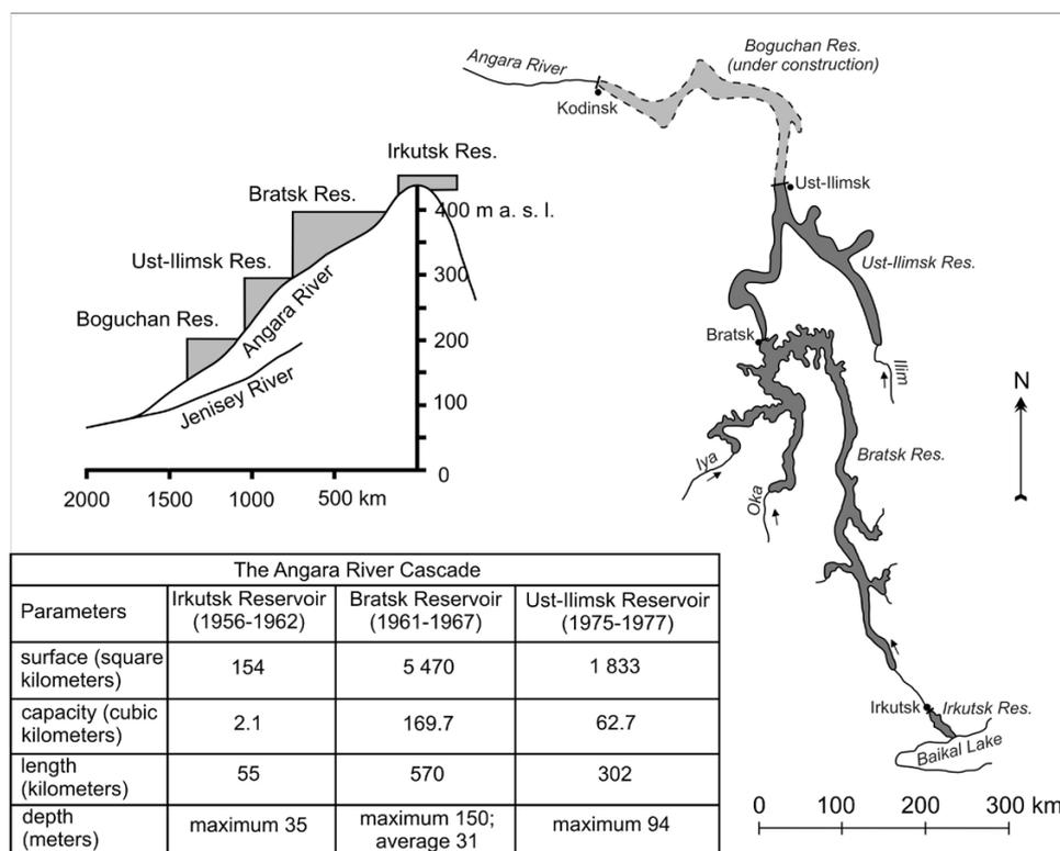
Fig. 1. The Angara reservoir cascade scheme, the main parameters
